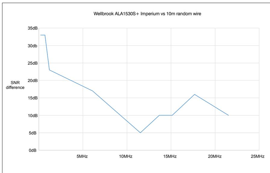
**Fig. 4:** A graph showing the performance of the ALA1530S+ Imperium versus a 10m random wire antenna.
